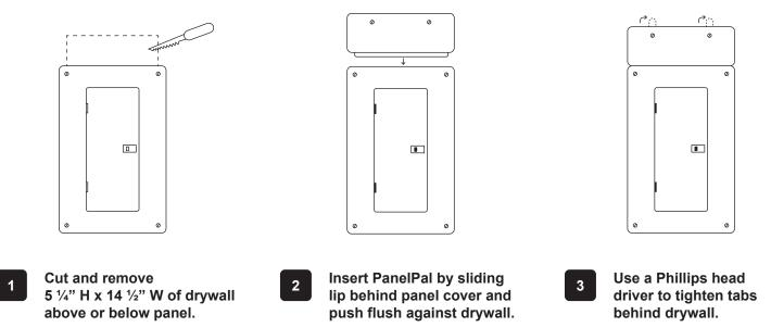
The Panel Pal is an innovative access panel installed above or below an electrical panel that eliminates the need for patching drywall. Use for adding a new circuit, change-outs, repairs, additions, renovations, upgrades, and more! **CAUTION:** Take safety measures when dealing with electricity. Turn power off to prevent injury.
